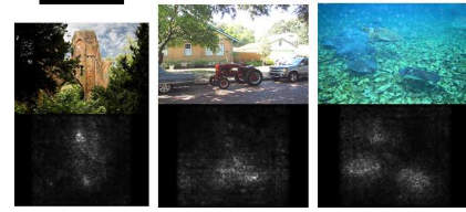
Fig. 8 Image-specific class saliency map for top-1 predicted class in ILSVRC-2013 test images. From [29] Fig. 2
